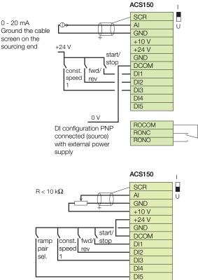
DI configuration NPN connected (sink)
