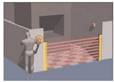
The worker gets out from the zone and presses the B button. He must do it in scheduled time to reset the machine.
