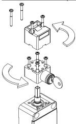
Before fixing the device, it is possible, if necessary, to adjust the position of the head and the key release device (if present) in order to turn the device to the position best suited to the application.
