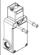
Attention: Always affix the device with 2 M5 screws with resistance class 8.8 or higher, flat seating heads and washers inserted beneath them. Install the screws with medium resistance thread lock, and a number of threads engaged equal to or greater than the screw diameter. The device must never be fixed with less than 2 screws.
