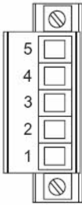
Fig. 10.3: Open-style plug on the MSI-FB-CANOPEN module
