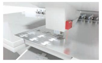
**Solution:** The ODSL 8 and ODS 9 sensors measure the distance with resolutions of up to 0.01 mm and thereby supply the basis for a high quality of this process step.
