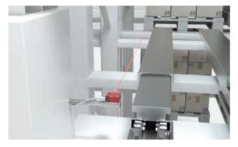
Solution: The ODS/HT 10, ODS/HT 110 and ODSL 96 sensors detect the pallet foot at a range of up to eight meters thanks to their focused laser. With switching product models, the movement of the pallet can be detected with the help of the window function.
