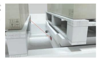
**Solution:** Thanks to their compact construction, the ODS / HT 10 and ODS / HT 110 sensors can easily be integrated in shuttles. Through time of flight measurement, the distance is detected independent of color.
