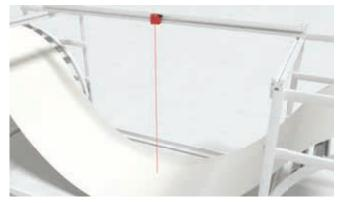
Solution: The tension of the material can be monitored by measuring the sag. Due to their various light-spot geometries, the ODSL 8, ODS 10 and ODSL 96 sensors can reliably measure the sag of a wide range of different material surfaces.
