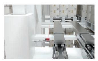
**Solution:** The ODS 10 and ODS 110 sensors can detect shelf racks at a distance of up to eight meters – independent of environmental influences.
