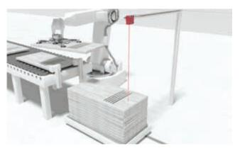
**Solution:** Our wide selection of distance sensors with various resolutions and operating ranges enables height measurement of different stacked objects.
