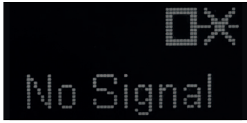
Fig. 8.7: Display: No measurement value in the case of deactivation
