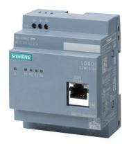
LOGO! CSM12/24 Compact Switch Module connection of a LOGO! (...0BA7/...0BA8) and up to 3 further nodes to Ind. Ethernet with 10/100 Mbit/s Unmanaged switch, 4 RJ45 ports, 1x front port for diagnostics DC 12/24V power supply LED diagnostics, LOGO! setup
