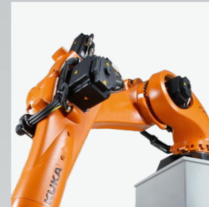
Robot knee positioned lower and further forward for greater downward reach.
