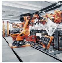
The KP1-HC500 welding a frame with its quick and precise alignment capability
