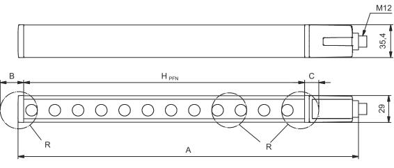
$H_{\mathsf{PFE}}$  Effective protective field height = 1540 mm  $H_{\mathrm{PFN}}$  Nominal protective field height = 1500 mm
